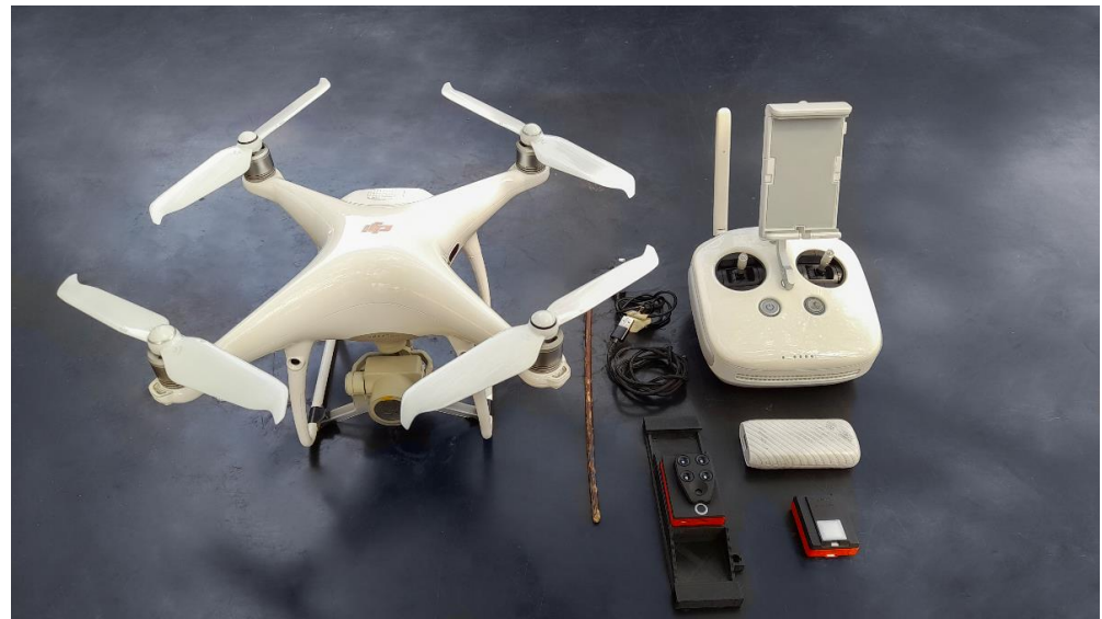
Figure 2. Equipment used in data collection. UAV and radio control, and Parrot Sequoia camera.
